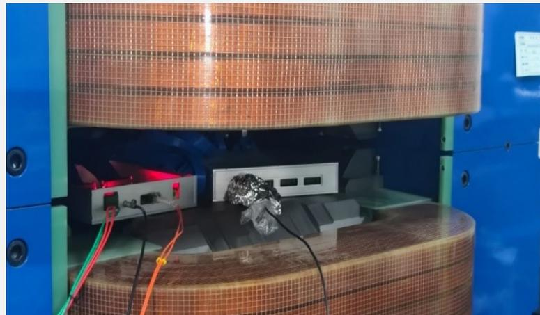
High magnetic field environment test
