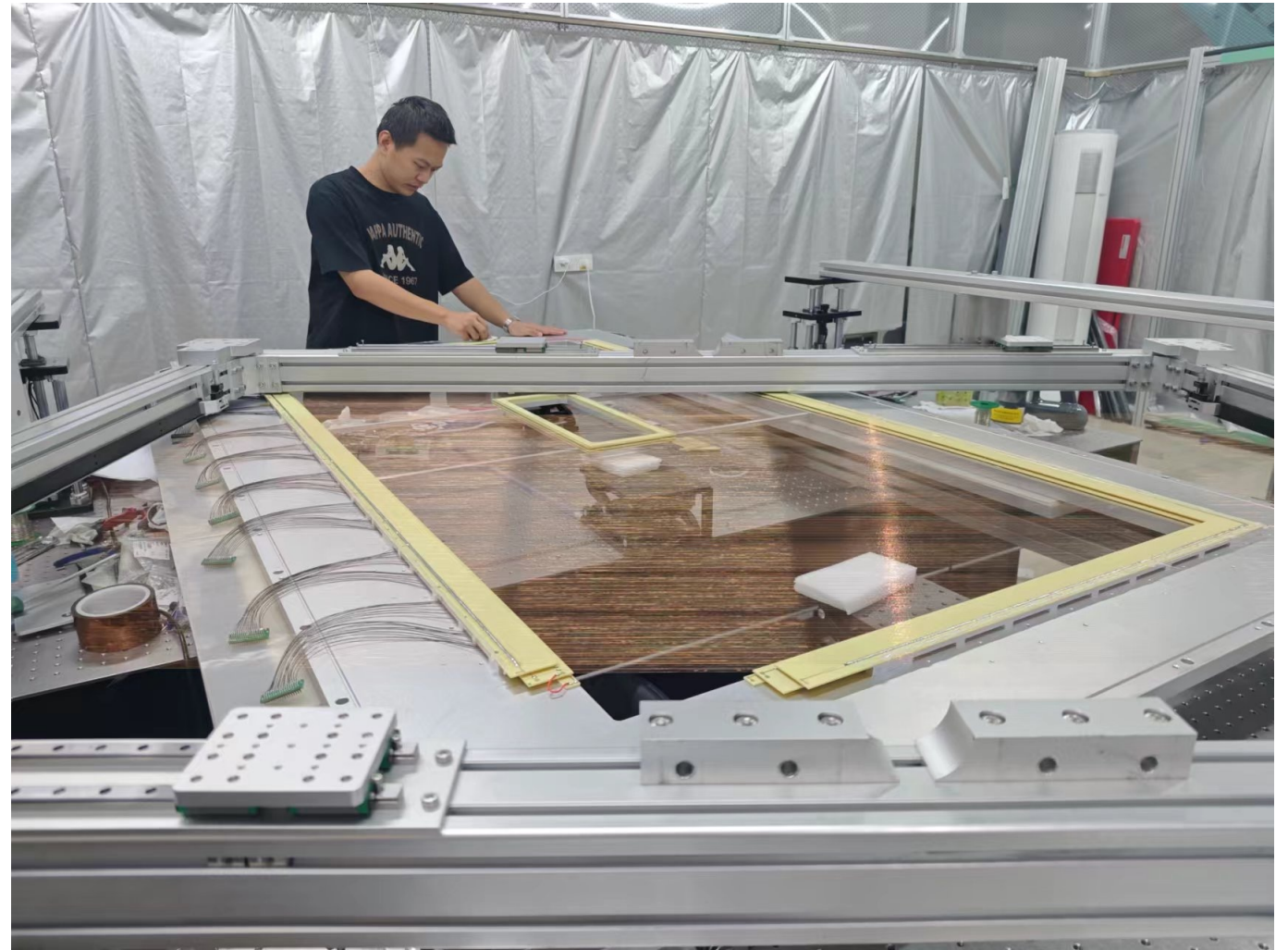
Wire alignment and welding operation platform
