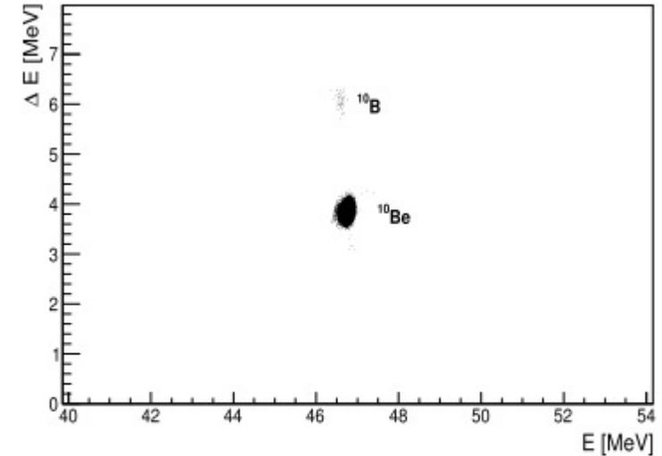
Fig. 4. DE-E spectrum measured, inside the CT2000 scattering chamber, with a telescope placed at zero degree hit by the  $^{10}\text{Be}$  beam with an intensity reduced to about 100 pps. The spectrum shows a pure  $^{10}\text{Be}$  beam with a minor  $^{10}\text{B}$  contamination of the order of 0.15%.
